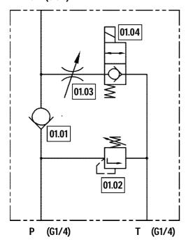
Port P is connected to port C through check valve 01.01. A leak-free closure is provided at port C by check valve 01.01 and directional poppet valve 01.04.
